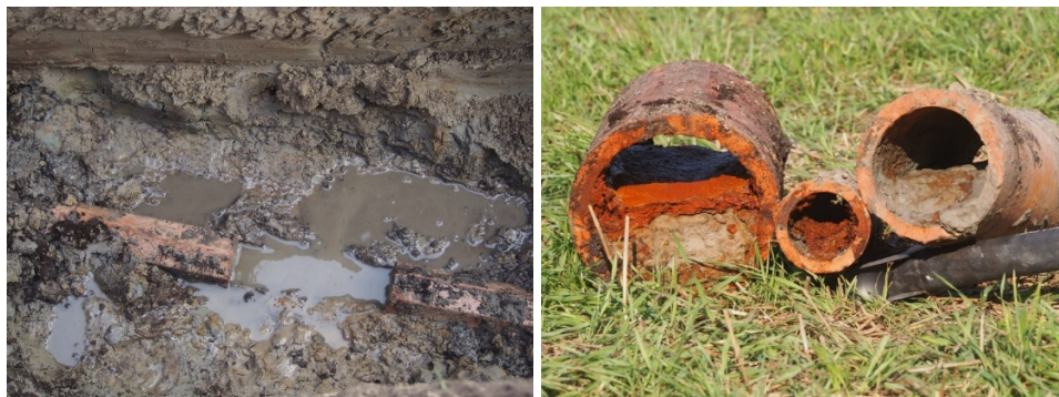
Figure 2. Silted drain pipes of different diameters
