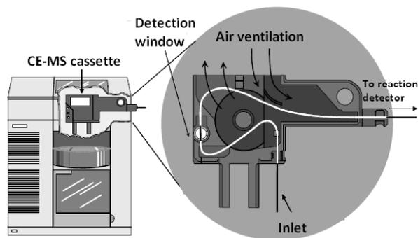
Fig.1. Scheme of capillary electrophoresis apparatus and standard mass spectrometry cassette (G1600-60013, Agilent Technologies, Germany), which was used for a development of on-line radical scavenging detection.
