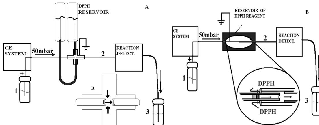
Fig. 2. The scheme of capillary electrophoresis – reaction detection setup: (A) with a stainless-steel cross connection interface and (B) funnel type interface. 1 – inlet vial (sample), 2 – reaction coil, 3 – outlet vial (waste). Sample is injected using 50 mbar pressure. This pressure is kept during the electrophoretic run.
