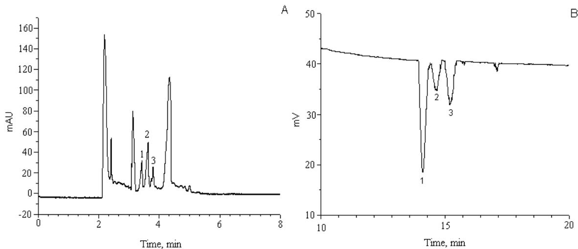
Fig. 3 (A) Electropherogram of the separated compounds of honey bees propolis aqueous extract obtained at UV wavelength 200 nm. (B) The DPPH• reaction detection signal profile at 517nm. Detector coupled on-line to the CE system. Reagent concentration 50µg/ml DPPH. Peaks1- ferulic acid; 2 - trans-p-coumaric acid; 3 - caffeic acid.
