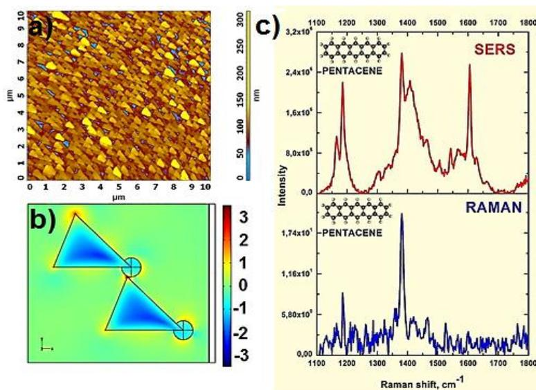
**Figure 1.** Silver nano-wedges decorated SERS substrate: a) AFM height image; b) theoretical model of electromagnetic field distribution of double wedge with a 5 nm gap:  $\text{Log}_{10}(|E|^2/|E_0|^2)$  in the X-Y plane at  $z=50$  nm; c) Raman and SERS measurements of pentacene monolayer evaporated on bare silicon wafer and SERS substrate.
